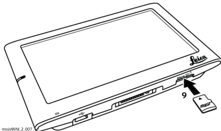
9. Insert the micro SD card into the slot at the bottom right of the mojoMINI 2.
