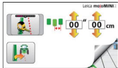
2. Select the desired lightbar mode by tapping the Lightbar Mode button until the button matching the mode appears.
