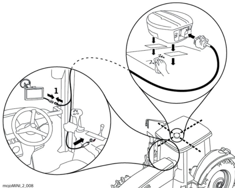
1. Connect the mojoMINI 2 cable to the grey square plug of the GeoSpective 2 smart antenna's cable.
