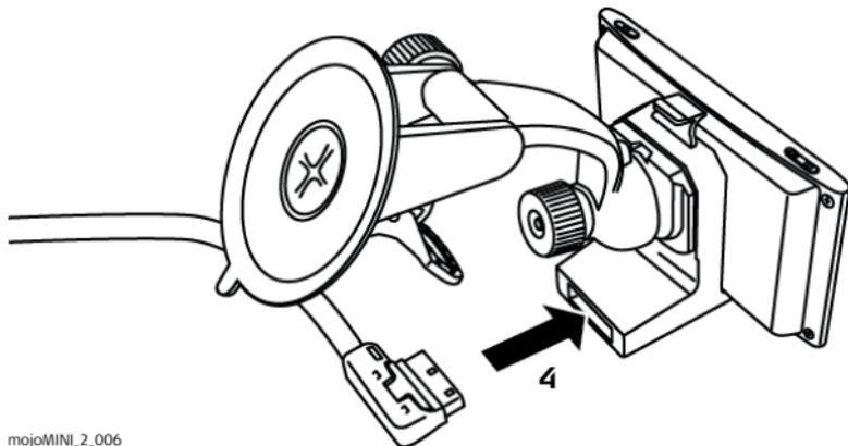
4. Plug the rectangular connector of the mojoMINI 2 cable into the socket of the mounting cradle.
