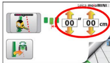
This setting determines how much crosstrack error is represented by each segment in the lightbar. A small number makes the lightbar more sensitive and hard to follow, but more accurate. A large number makes the lightbar less sensitive and easy to follow, but less accurate. This value has a range of 0.4"/1cm to 8.0"/20cm per segment.
