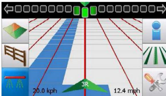
The main navigation screen has five main parts: the lightbar, main display, information area, left menu bar and right menu bar.
